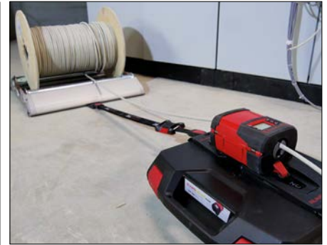
RUNPOMETER RM35 with connecting pad and belt fixed to cable drum roller PRO
