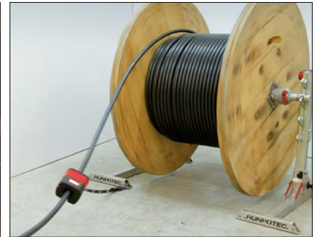
RM35 with RUNPOLIFTER L1600 and 3 x 35 mm² cable
